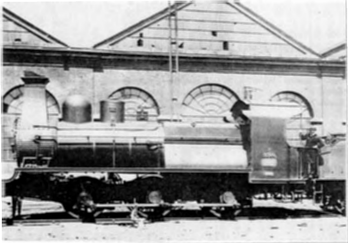
Type 25. With square chimney later modified to a cylindrical shape, as seen on CF 307
